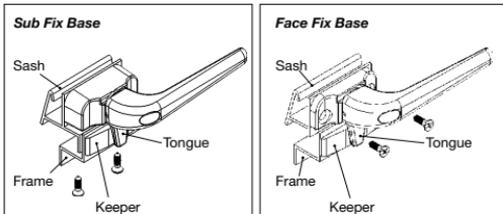
**1A** Remove existing handle by unscrewing fixing screws or drilling out the head of the rivets if used
