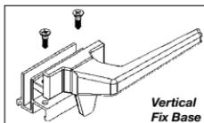
**2B** Locate the conical points of the "marking gauge" provided in the existing holes ensuring that the arrows point to the glass. Mark the position for the new holes through the holes in the "marking gauge". Centre punch the new hole positions before drilling using a 3.5mm drill
